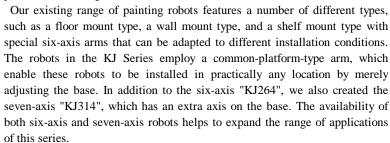
The arm of the KJ Series is both lighter and thinner than existing models. The cabling is also housed within the body of the robot, allowing for multiple
