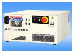
large-capacity, compact power unit that can accept power from a single phase 200V input, enabling the "YF03N" to accelerate rapidly. Functional safety technologies are employed that eliminate the need for electromagnetic contactors, thereby making the product more reliable. The "E9\*" controller can also be used with the "YS02N", the new picKstar model, to provide the production line with more flexibility and help save space.
