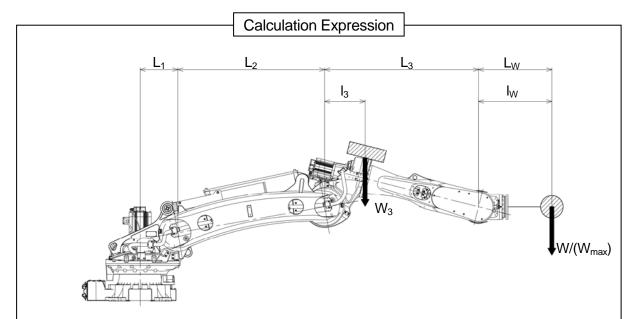
W<sub>max</sub>: Max. allowable load [kg]
