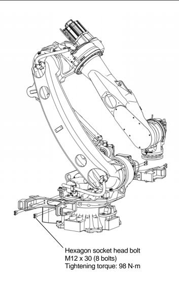
Remove the fork pocket attached to the arm once the transportation of robot is complete.
