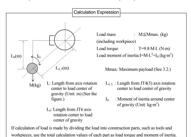
Regarding the load on the robot wrist section, meet the following restriction conditions:
